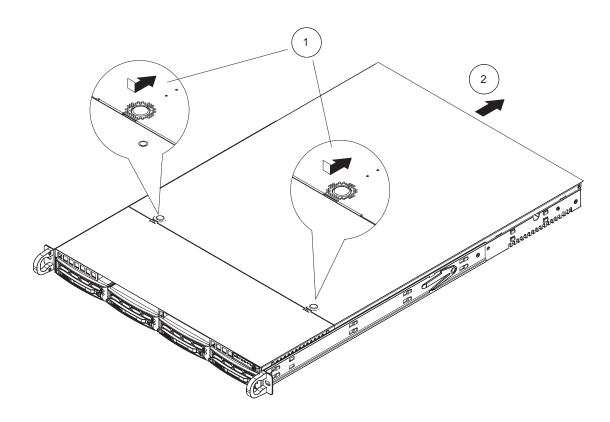
Figure 2-5. Accessing the Inside of the System
